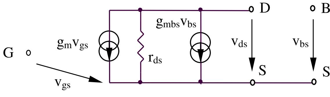
$$g_m = \frac{\partial I_D}{\partial V_{GS}}$$
