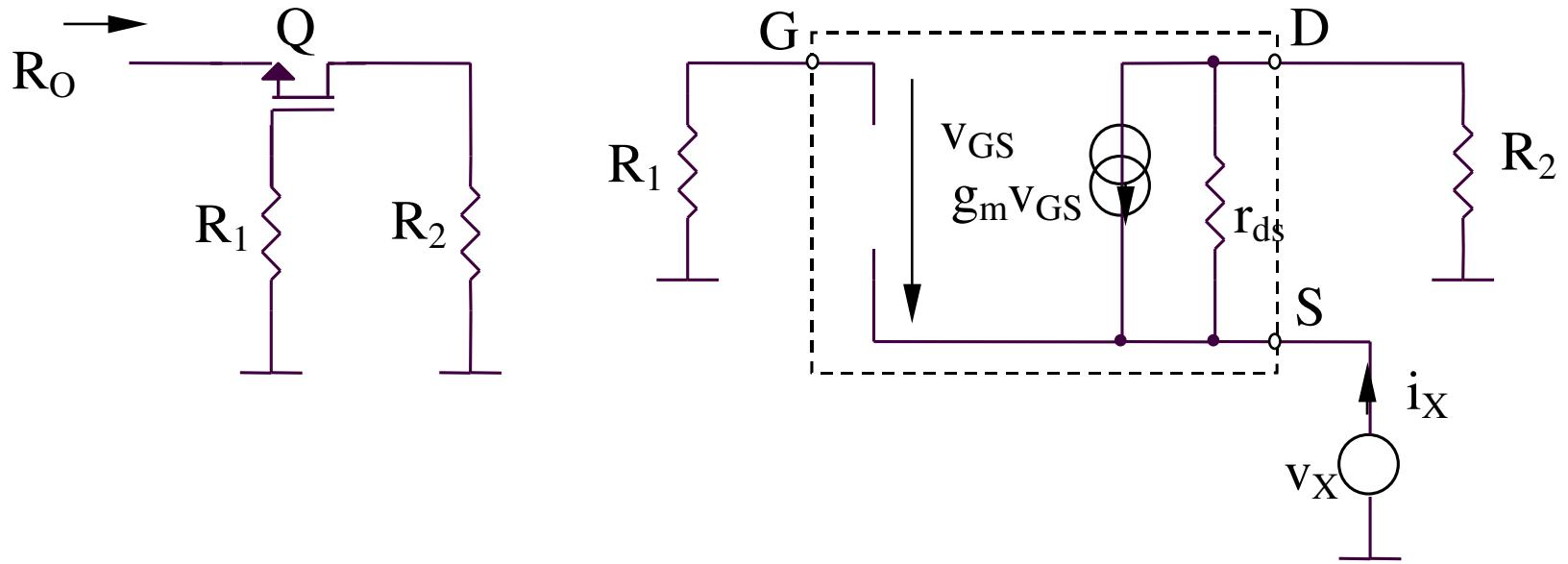
$$i_x \cong -g_m v_{gs} = g_m v_x \Rightarrow R_O = \frac{v_x}{i_x} = \frac{I}{g_m}$$
