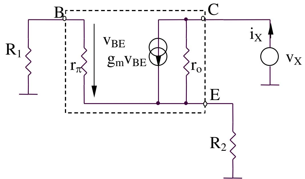
$$R_O = r_o \left( 1 + \frac{\beta R_2}{r_\pi + R_1 + R_2} \right)$$
