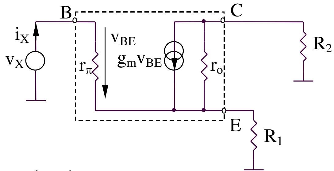
$$v_x = i_x r_\pi + (\beta + 1) i_x R_1$$
