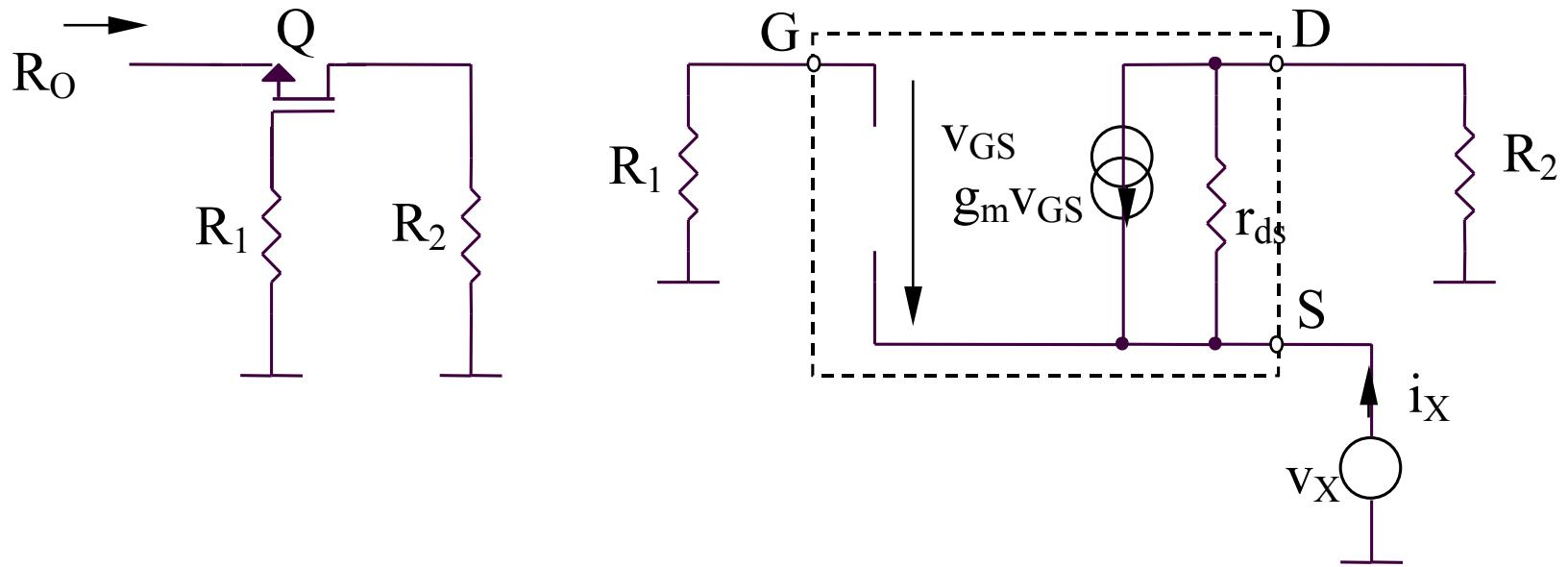
$$i_x \cong -g_m v_{gs} = g_m v_x \Rightarrow R_O = \frac{v_x}{i_x} = \frac{1}{g_m}$$
