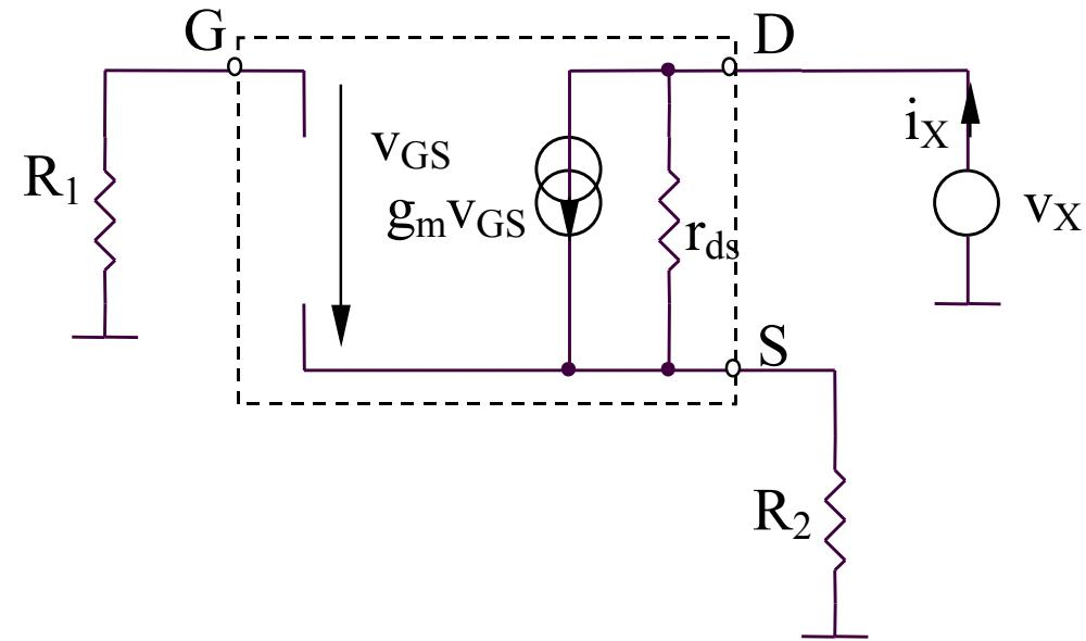
$$\left. \begin{array}{l} v_x = (i_x - g_m v_{gs}) r_{ds} + i_x R_2 \\ v_{gs} = -i_x R_2 \end{array} \right\} \Rightarrow R_O = \frac{v_x}{i_x} = r_{ds}(1 + g_m R_2) + R_2 \cong r_{ds}(1 + g_m R_2)$$
