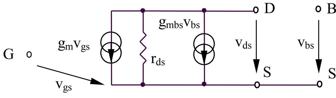
$$g_m = \frac{\partial I_D}{\partial V_{GS}}$$
