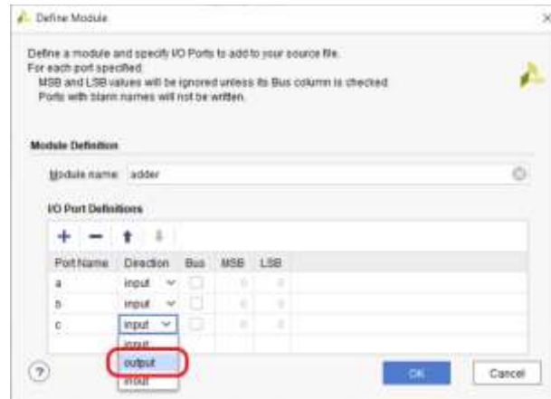
Figure 19: Define module window, change a port direction
