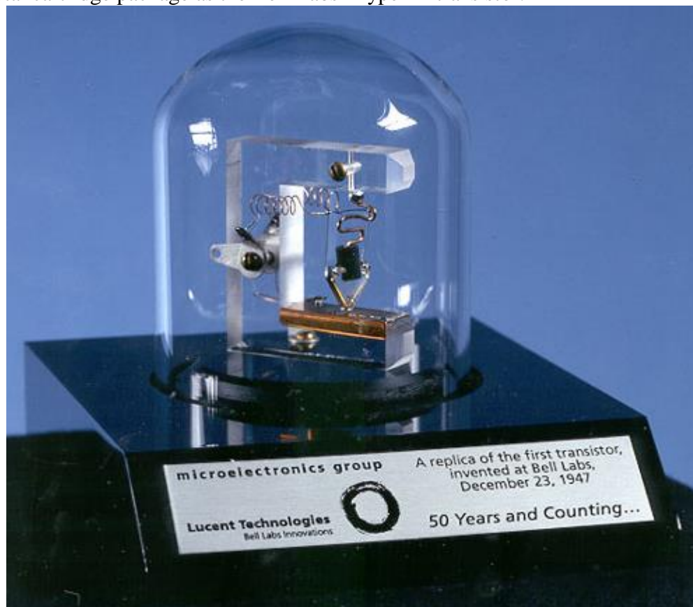
Fig.1. A replica of the first point-contact germanium transistor, Bell Labs (Lucent-Nokia)
